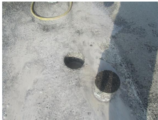
Figure 1. Obtaining the asphalt coring samples
