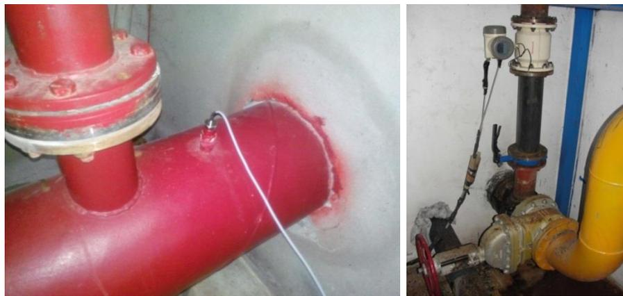
**Figure 5.** Temperature measurement at the inlet of the transmission pipeline (left), flow rate measurement at the outlet of the transmission pipeline (right).
