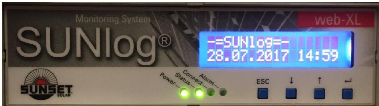
**Figure 4.** Data logging unit for PV system.
